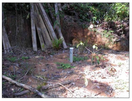
Figure 11.3 Drill-hole Collar Marker
